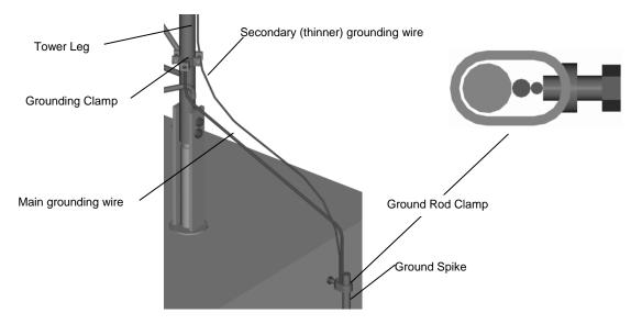
Figure 2-12 Grounding the Datalogger and the Tower
