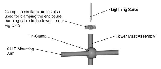
Figure 2-1 Attaching the Lightning Spike
