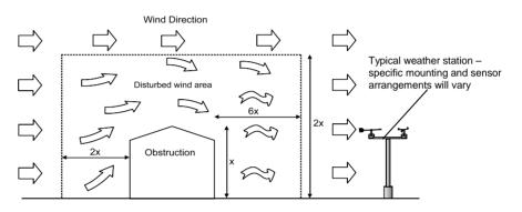
Figure I-1 Effect of Structure on Air Flow
