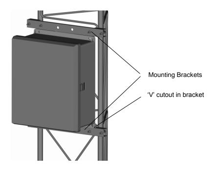
Figure 2-10 Fitting the Enclosure
