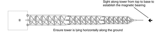
Figure 2-4 Sighting Along the Tower to Check the Magnetic Bearing
