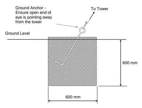
Figure 1-6 Ground Anchor Installation
