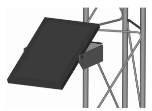
Figure 2-11 Fitting the Solar Panel
