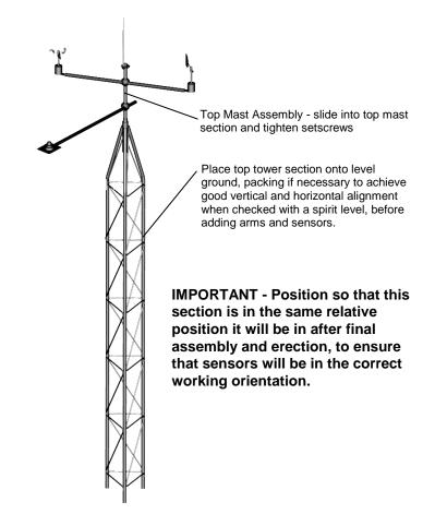
Figure 2-2 Top Tower Section at Ground Level
