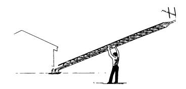
Figure 2-8 'Walking' the Tower into the Upright Position
