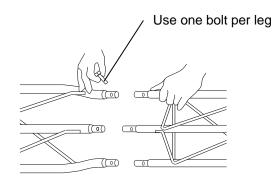
Figure 1-7 Fitting the Tower Sections
