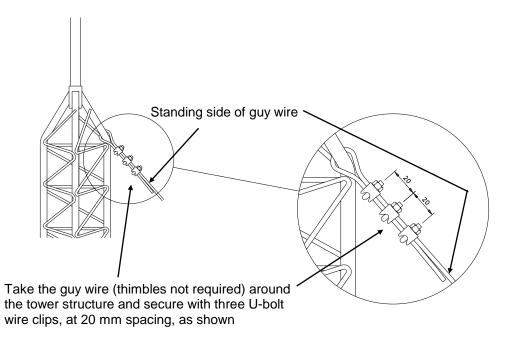
Figure 2-7 Installation of Guy Wires to Tower
