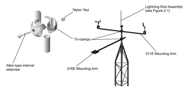
Figure 2-6 Both Mounting Arms and Sensors in Final Position on the Tower Mast Assembly
