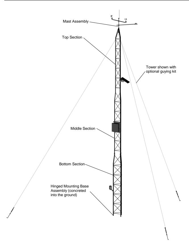
Figure 1-2 UT30 Tower Assembly, with Enclosure, Solar Panel and a Typical Range of Sensors
