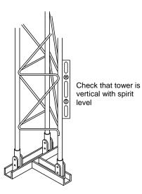
Figure 1-4 Special Roof-Mounting Base Installation for UT30
