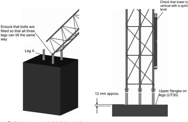
To tilt the tower, remove both bolts from leg A. (see above). Remove the lower bolts and loosen the upper bolts in the other two legs.
